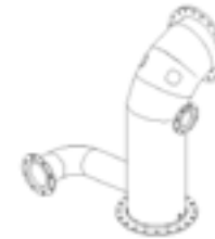
Water injection piece for a main engine, including relatively large bypass pipe.
